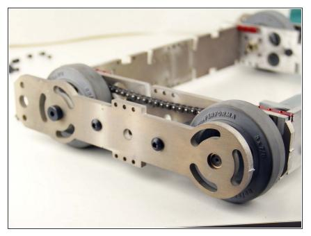
Now use the 1/4"-20 button head screws to fasten the outer frame rail to the standoffs
