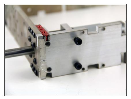
Using 10-32 socket cap screws, thread in and loosely tighten to secure the gearboxes' additional mounting points.
