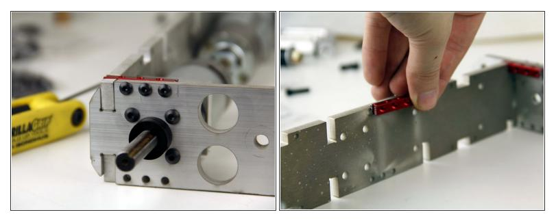
• Time to insert all the nut strip blocks and 6-32 button head screws
